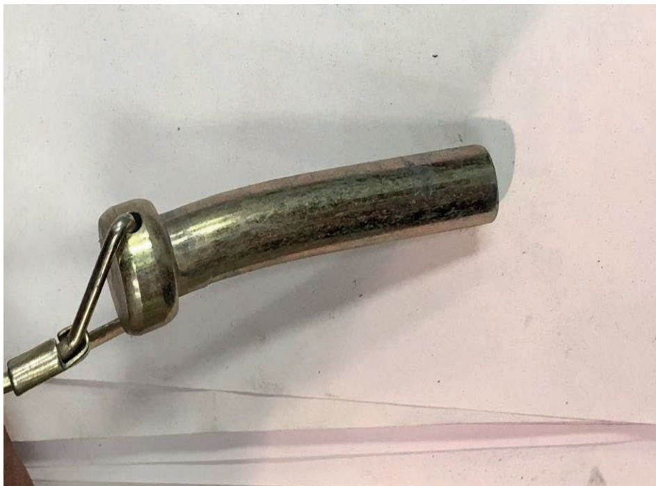
Digital image showing securing pin deformation, post load application.
