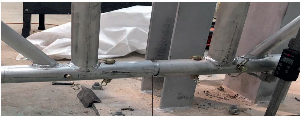
Tension through lower chord under load condition
